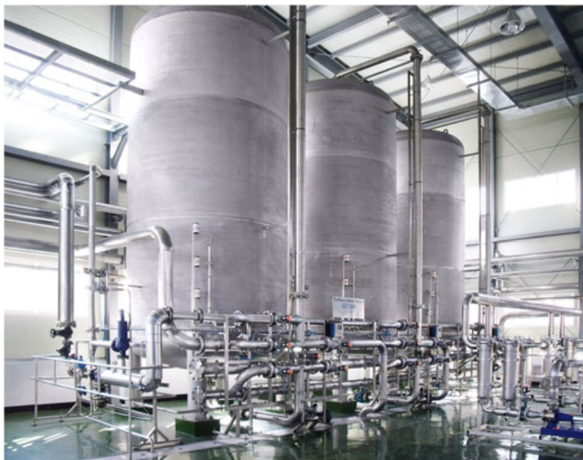
Figure 10. Activated carbon filtration in Korea, 285 \text{ m}^3 \text{ h}^{-1} (by EUWA).
