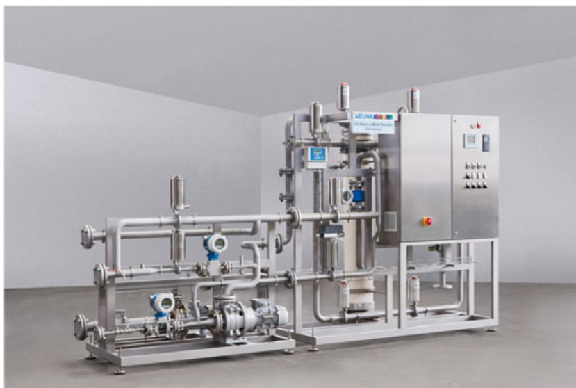
Figure 11. Membrane-based lime water production in Germany, 500–1500 l h -1 (by EUWA).
